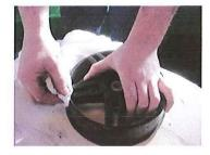
Prepare the wheel centre for fitting the new tyre by removing any dirt which may have collected on the hub.
