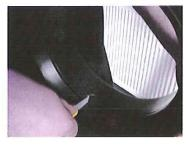
Ensure the tyre is smooth inside. This may require the inside joint line of the moulding to be trimmed if it has not already been trimmed, as this will prevent the tyre snap fitting to the wheel centre.
